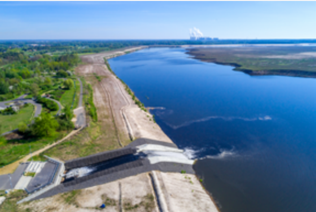
Picture 5: View of the northern area of the Cottbuser Ostsee lake with the inlet structure in May 2021. First, the deeper border cuts of the former opencast mine are filled by the water. Later, the water will cover the large inner dump area, too.
